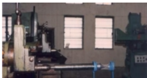
Fig. 1 Trouble testing set-up for mandrel test
